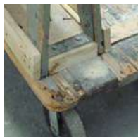
Wood—splinters and rots
